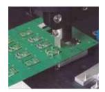
Two standard drop in die sets are available. The first is a two pin die set which allows the operator to bring the pins to the correct position for setting the edge of a round panel to center under the cutting line of the blades. The second drop in die is for panels which may need more positioning pins than a standard round or square panel. This provides a flexible positioning platform for many different panel geometries.
