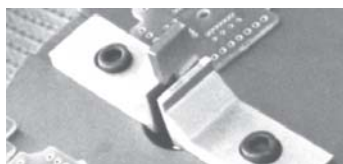
Sharp double knife support die for clean tab cut off.
