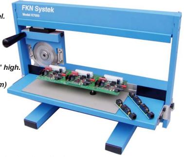
**The K7000** is a circular linear blade depanelizer developed to singulate prescored PCBs with very tight component spacing. The linear blade is 12" (304mm) long and has a .030" (.762mm) thin symmetrical cutting edge designed particularly for PCBs with closely spaced components.
