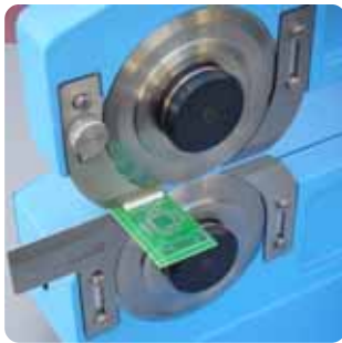
Adjustable front blade guard. Only scoreline can pass to cutting blade.
