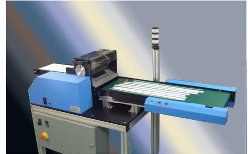
In line PLC controlled K5000 accepts PCBs from output conveyor of solder re-flow line via SMEMA interface.
