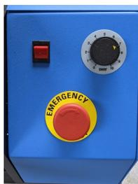
The operator fed version of the K5000 has a simple control panel with on/off switch, speed control and E stop.
